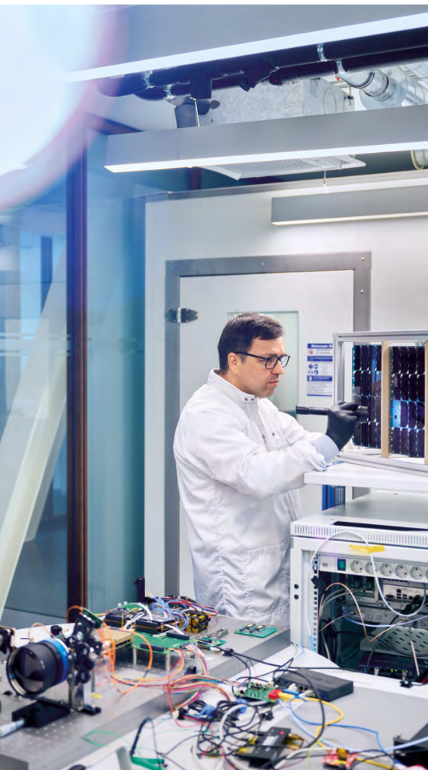
Prof. Frank Schäfer working in earnest on ERNST: Before ERNST, Fraunhofer's own research satellite, goes into space in 2024, it will first undergo top-to-toe testing at the Fraunhofer EMI laboratory in Freiburg — here, the solar module is being checked.
