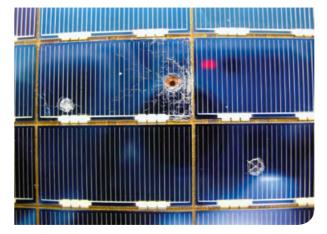
Damage to the Hubble space telescope, which was launched into orbit in 1990. © *ESA*
